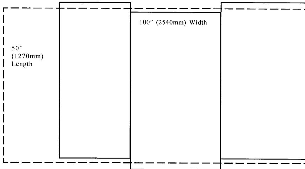
**\*\* Note that the Standard is 99/100" (2515/2540mm) Width X 50" (1270mm) Length. Diagram shows 100" (2540mm) only.**
